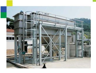
Flow ranges vary according to each particular case (application, suspended solid concentration, etc.), but ECOTEC can deliver equipments for flows up to 300 m<sup>3</sup>/h per unit.
