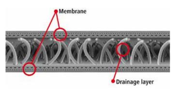
Especially when considering wastewater treatment using MBRs the integrity of the membrane plays a significant role. The actual cleaning of the wastewater in the MBR process is being performed by the biomass in the system. The membrane used must now ensure the safe separation of the biomass from the cleaned wastewater. Superficial damages to the membrane should therefore not compromise this.
