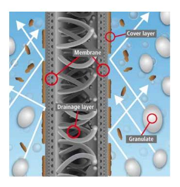
This mechanical cleaning can only be used in conjunction with BIO-CEL® modules, because other module types do not incorporate the required constructional and hydraulic characteristics to perform a mechanical cleaning.
