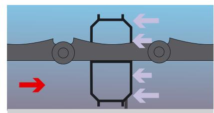
The forces above and below the chain balance each other, causing the chain to run without any vibration and significantly reducing the chain's wear in the flight attachment.
