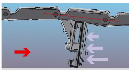
In traditional scraper flights, the pulling alignment is up. The flight is exposed to vibration, which causes the chain to wear.
