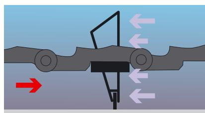
By lowering the chain's attachment point to the middle of the flight, the caused by vibration can be removed and the flight will run evenly.
