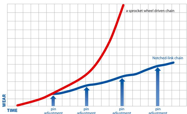
The drive pin adjustment performed during basic maintenance increases the life time of the chain and wheel.
